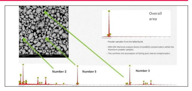
The image in the top left shows two brighter particles in this sample of material. The chart in the top right of the slide shows the analysis for the overall area of the powder whereby it detects Aluminum, Silicon and Magnesium as you would expect for the material.
